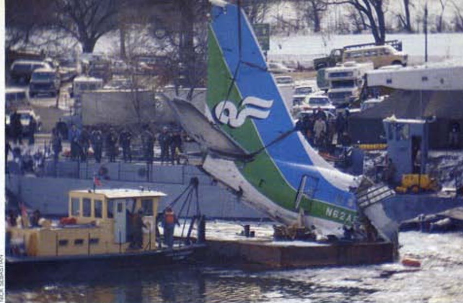
The tail section of the Air Florida plane fell back into the river during the first try by recovery teams to lift it from the river, but it eventually was loaded onto a barge and trucked to a hangar at National Airport, where it was examined by federal investigators. All the survivors were seated near—either just behind or just in front of—where the tail sheared off from the fuselage.
